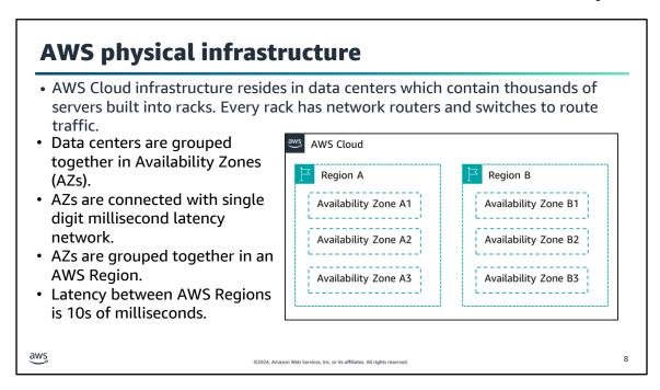
When you design your network on AWS, you need to understand the AWS physical infrastructure components and hierarchies. The AWS physical infrastructure is made up of multiple AWS Regions. Each AWS Region is a separate geographic area located in a country.
