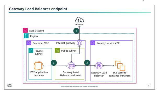
**Image description:** VPC 1 has a private subnet containing an EC2 instance and a public subnet with an attached Gateway Load Balancer endpoint and an internet gateway. VPC 2 has a Gateway Load Balancer and a EC2 security appliance instance. **End of image description.**
