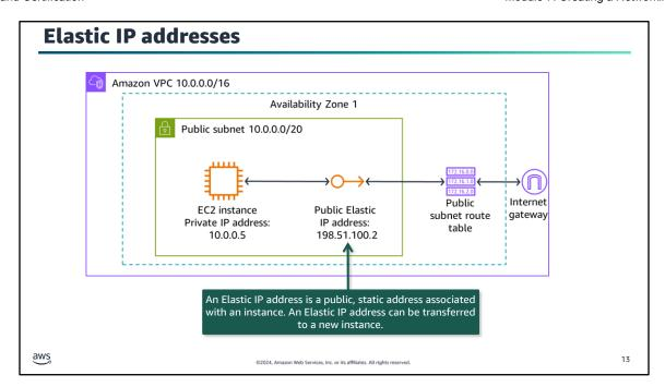
An Elastic IP address is a static and public IPv4 address that you can associate with an EC2 instance. If the EC2 instance's health deteriorates, you can transfer the Elastic IP address to a new, healthy EC2 instance. An EC2 instance private IP address is dynamic as it is released when the instance is terminated.
