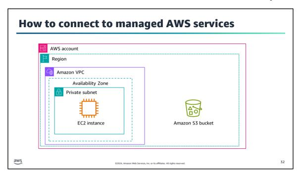
**Image description:** Architectural diagram of an AWS VPC with an EC2 instance in the private subnet. An Amazon S3 bucket using separate Gateway VPC endpoint. The EC2 instance can access other AWS managed services and Amazon S3 using an interface VPC endpoint. **End of image description.**
