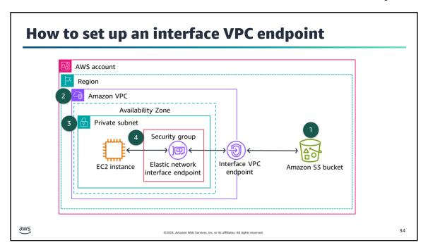
**Image description:** Architectural diagram of an AWS VPC with an interface VPC endpoint. The VPC contains a private subnet with an elastic network interface. The EC2 instance inside the private subnet can Amazon S3 using the network interface belonging to the interface VPC endpoint. **End of image description.**
