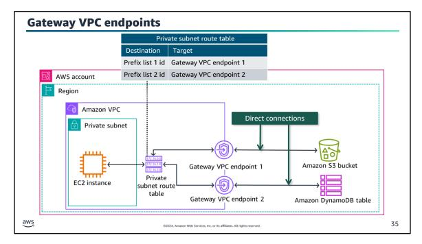
**Image description:** Architectural diagram of an AWS VPC with two gateway VPC endpoints. The EC2 instance in the private subnet can connect to Amazon DynamoDB and Amazon S3 each using separate gateway VPC endpoints through a private subnet route table. **End of image description.**
