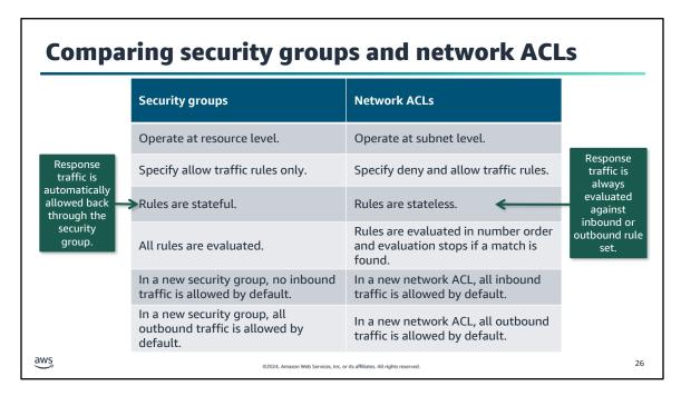
It's important to note the differences between security groups and network ACLs. Security groups operate at resource level while network ACLs operate at subnet level. Security groups only specify allow traffic rules while network ACLs specify deny and allow traffic rules.
