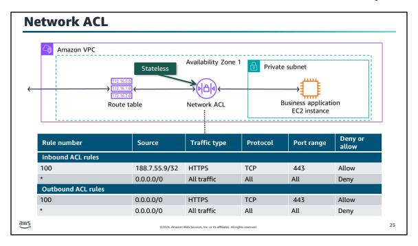
A network access control list (network ACL) is an optional layer of security for your subnet. It acts as a firewall for controlling traffic in and out of one or more subnets. To add another layer of security to your subnet, you can set up network ACLs with rules in the same way that security group rules are set up.
