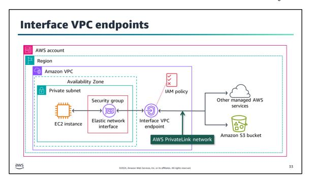
**Image description:** Architectural diagram of an AWS VPC with an interface VPC endpoint. The VPC contains a private subnet with an elastic network interface. The EC2 instance inside the private subnet can access other AWS managed services and Amazon S3 using the elastic network interface belonging to the interface VPC endpoint. The interface VPC endpoint has an IAM policy attached. **End of image description.**
