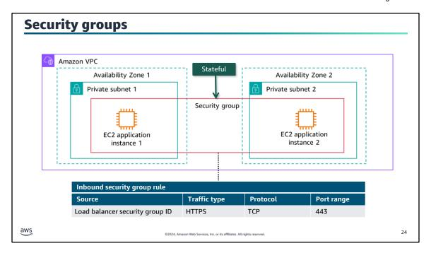
Security groups are stateful firewalls that act at the level of instance or a network interface. They can span can span multiple AZs. For each security group, you add separate sets of rules for inbound and outbound traffic. Resources with the same security requirements should be grouped together in one security group. In this example, business application instances across multiple AZs are associated with the same security group.
