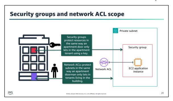
Security groups and network ACLs both are mechanisms that allow you to define network traffic filters called rules. Both can be used simultaneously, or only one can be used. Think of it as a person that lives in a high rise apartment in a big city.
